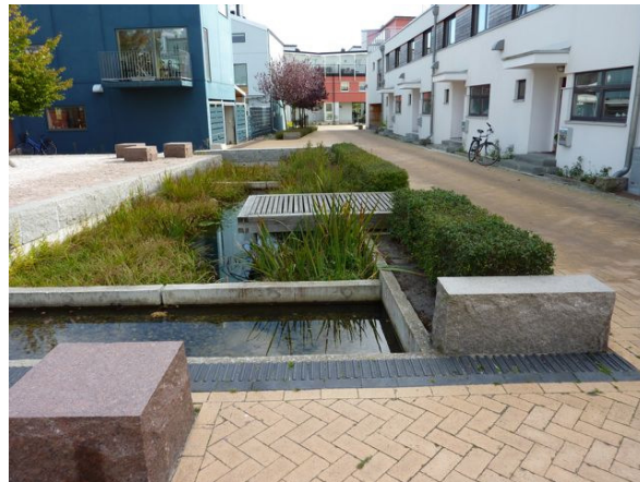
Figure 12 - open drains feed landscaped areas and ponds
