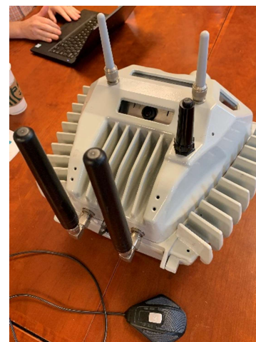
Figure 27 – Traffic safety sensors
