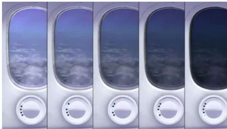
Figure 43 – Electrochromic windows – Boeing 787 Dreamliner
