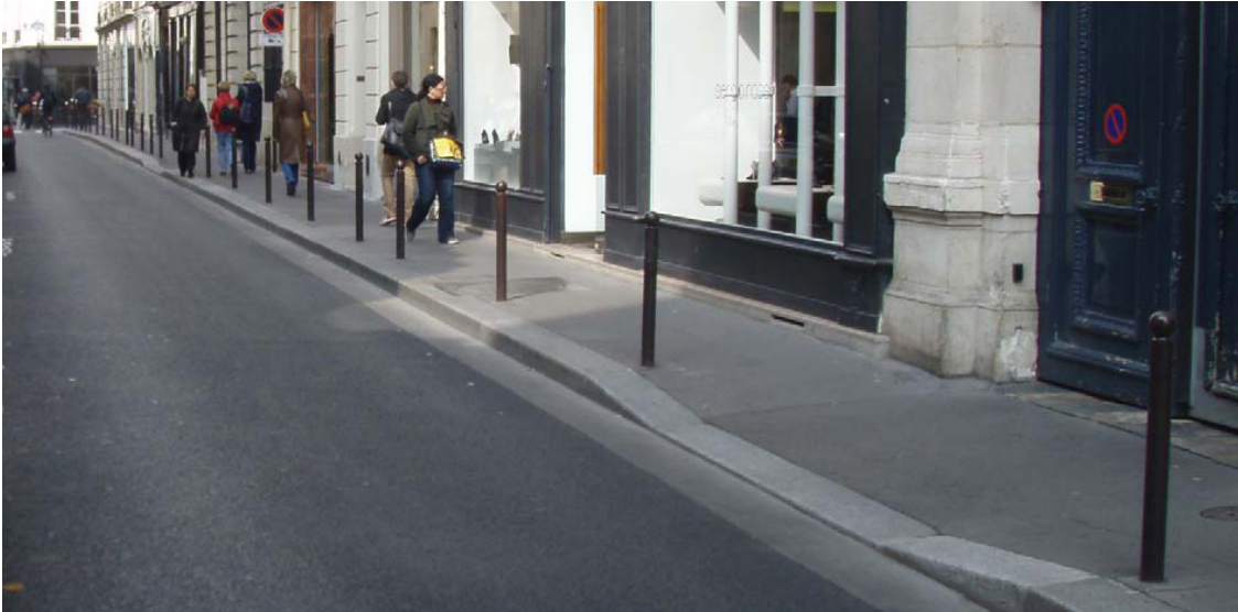
Figure 4-8: Footpath Protection / Guidance Treatment - Paris, France
